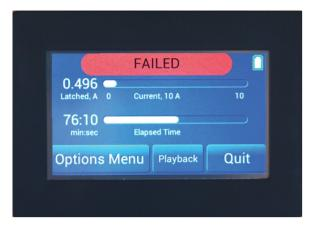
The Parasitic Drain Tester, **PDT Heartbeat 1001**, is an automotive diagnostic tool used to conclusively determine if a vehicle, motorcycle, RV or other 12 volt system has an excessive
